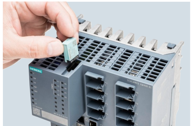
Plugging the C-PLUG into the SCALANCE XM408-8C switch
