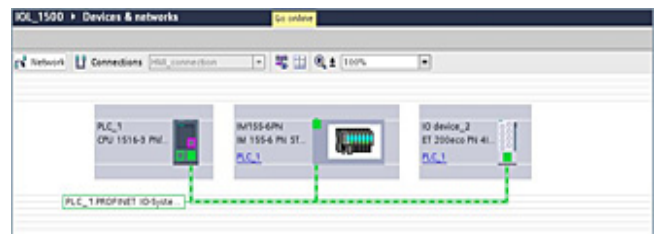
Configuration of a PROFINET network with lower-level IO-Link masters
